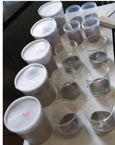
Figure 43. Samples to determinate density of ashes
