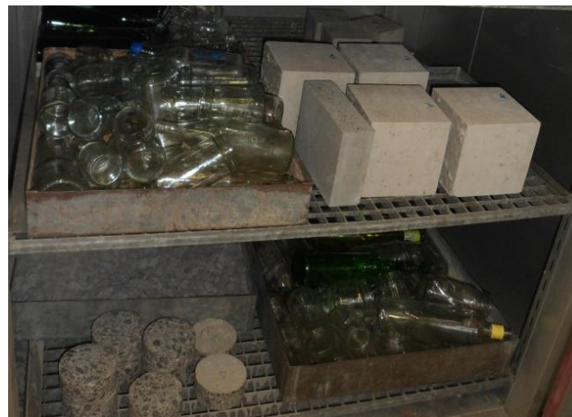
Figure 30. dry bottles in the oven 105°C
